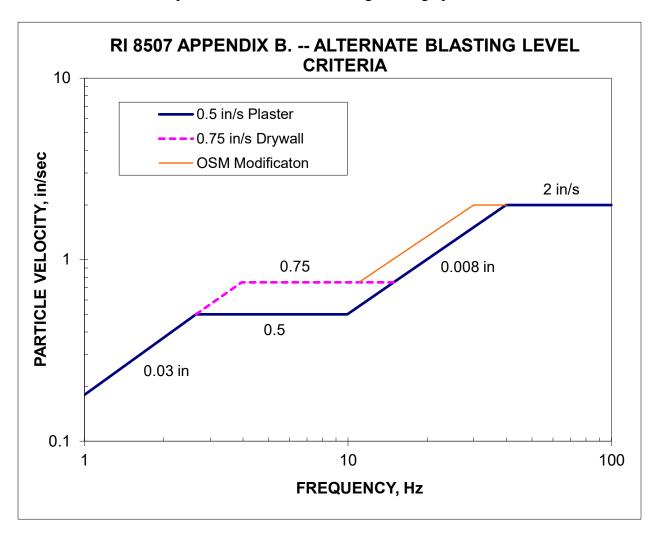
Figure B – 1. – Safe levels of blasting vibration using a combination of velocity and displacement
