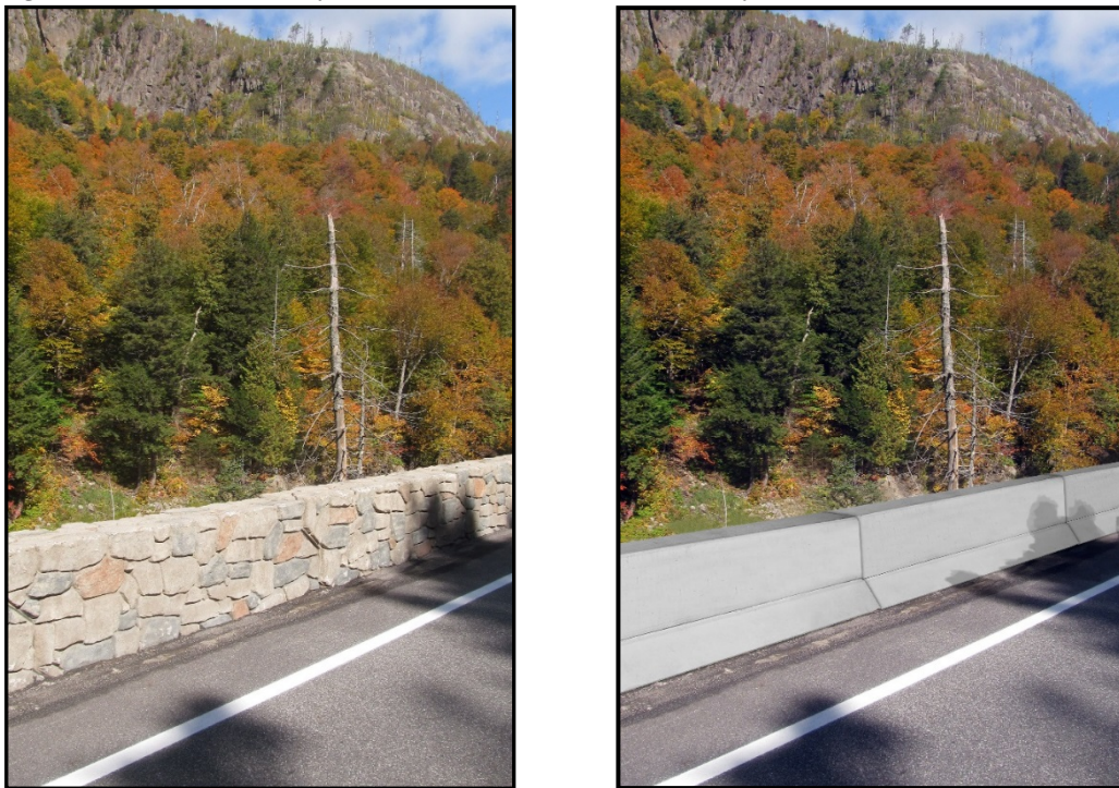
Figure 4.31 Simulation of Jersey Barrier with and without Adirondack Drystack Texture and Color
